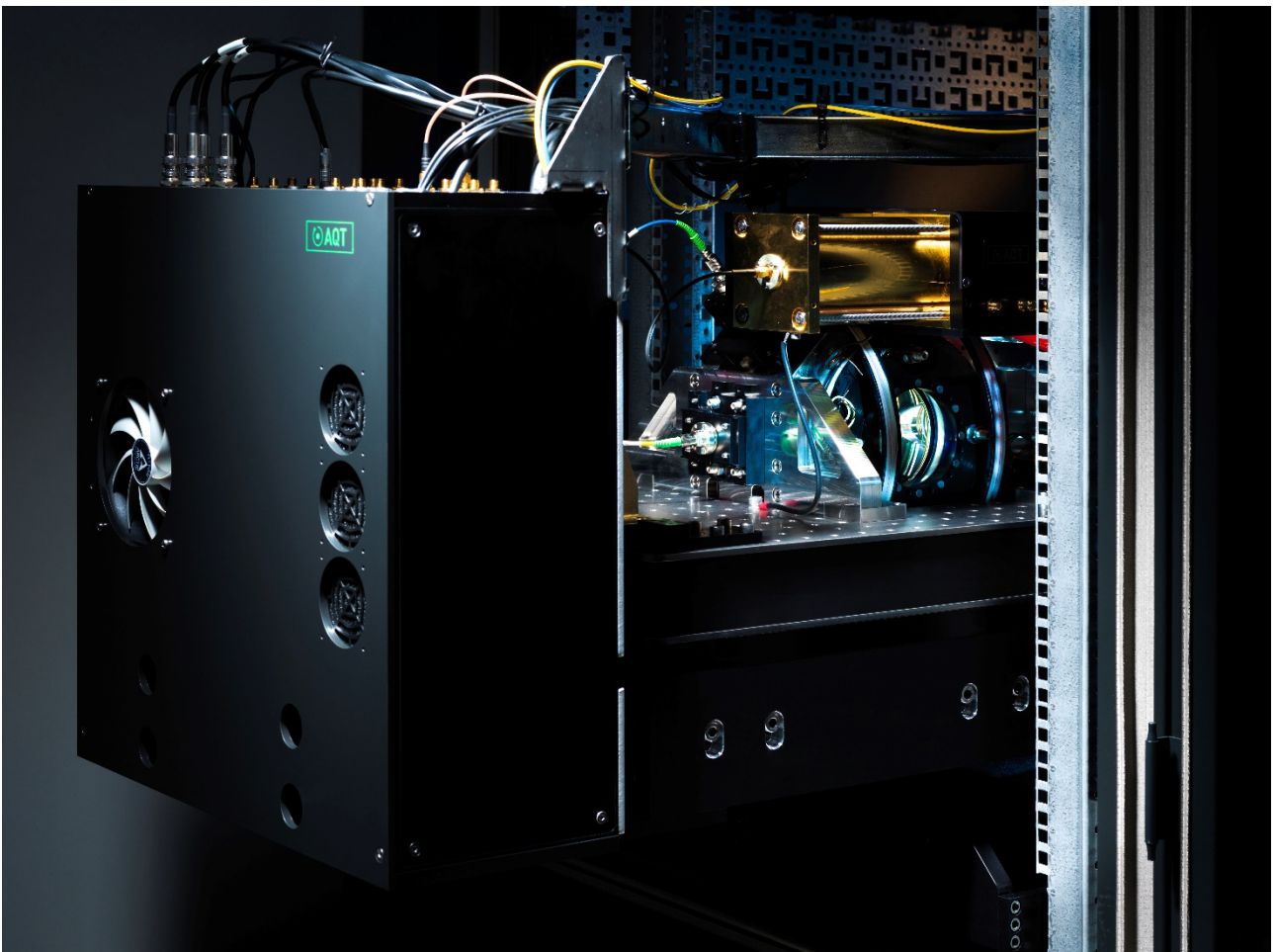
Image 2: Rack-mounted ion-trap quantum processor Photo: Dieter Kühl
